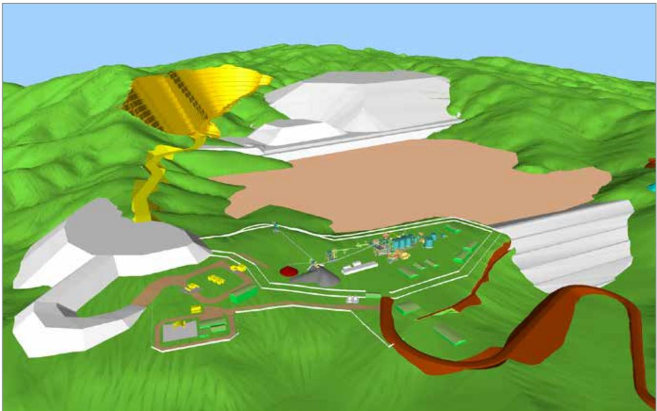
*Mako mine site infrastructure, including open pit, Waste Rock dump, Tailings Facility, Rom Pad, Processing plant and Mine services Area*
